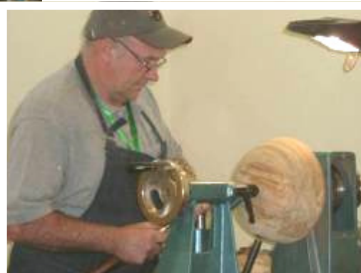
◀ Tony Rea gives a multitude of tips for dealing with spalted beech, including glueing a waste block on the bottom of a bowl to have a stable point to chuck on to.
