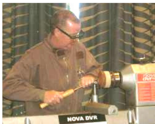
Stuart Mortimer demonstrates his ► method of lighting the inside of a hollow form to ensure an even wall thickness.
