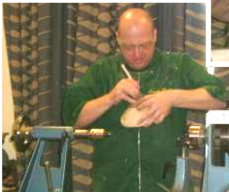
Mark Baker gives demonstrates the use of bowl gouges and scrapers. ▼
