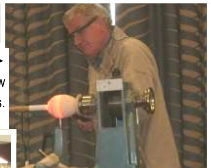
◀ Tony Rea gives a multitude of tips for dealing with spalted beech, including glueing a waste block on the bottom of a bowl to have a stable point to chuck on to.
