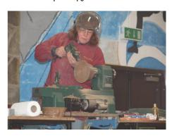
The top edge is cleaned up with a razor sharp gouge, and sanded with 240 grit. At this point the ceramic disc recess is finally sized. Christien suggests focusing on the opposite side to the point of cutting. "It gives you a better sense of what's happening. Have patience, and remember that an increment of, say 1mm at the tool is 2mm on the recess!"
