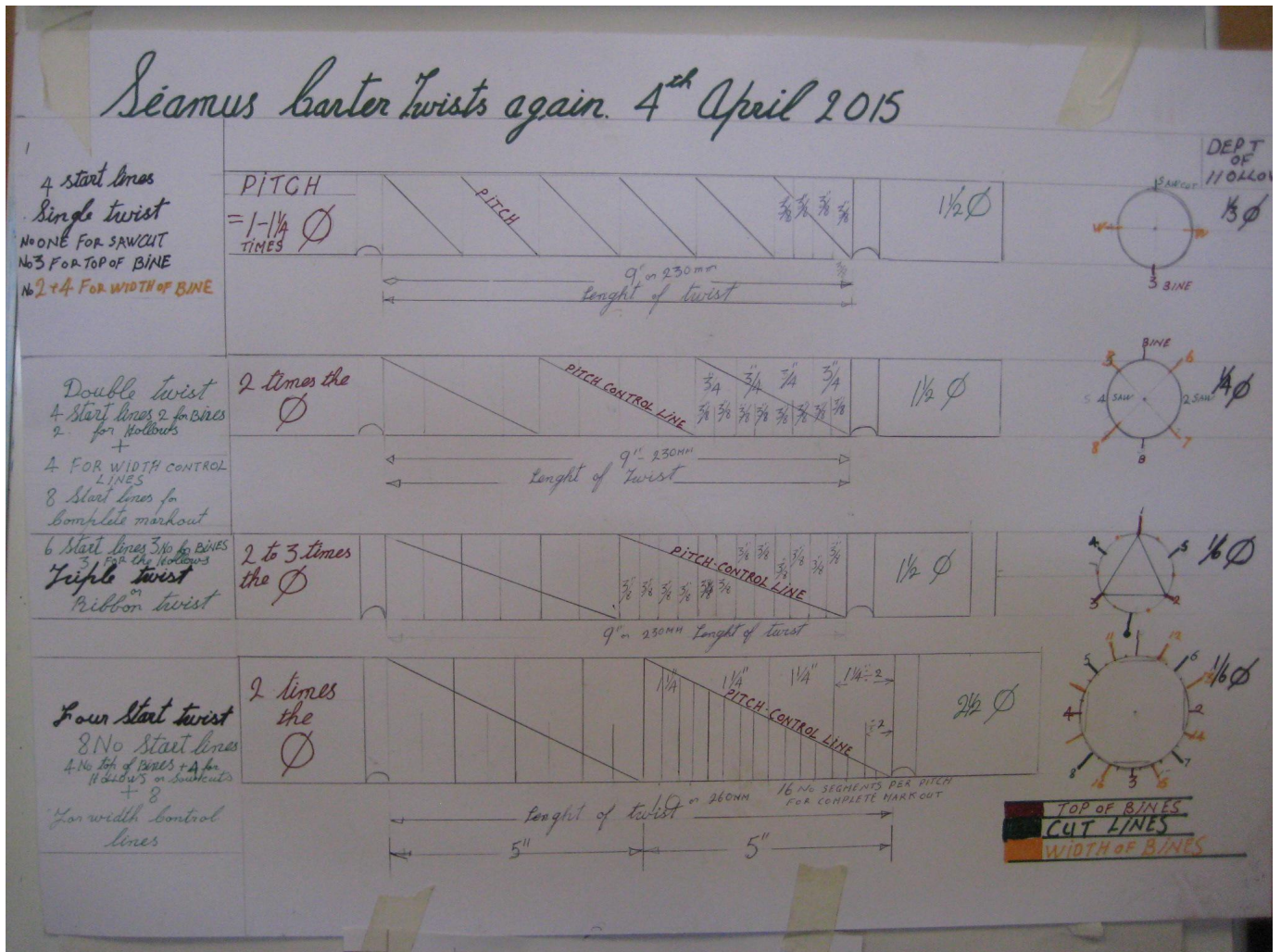
Above is a chart used during Seamus Carter's April demo, explaining everything you need to know an about marking out barley twist pieces.
