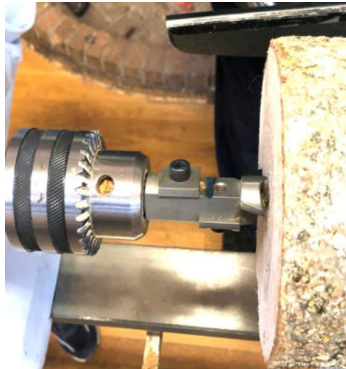
pic left variable width drill bit pic right cabide hollowing tool in action
